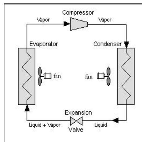
**Figure 4.** System Process Diagram <sup>7</sup>
