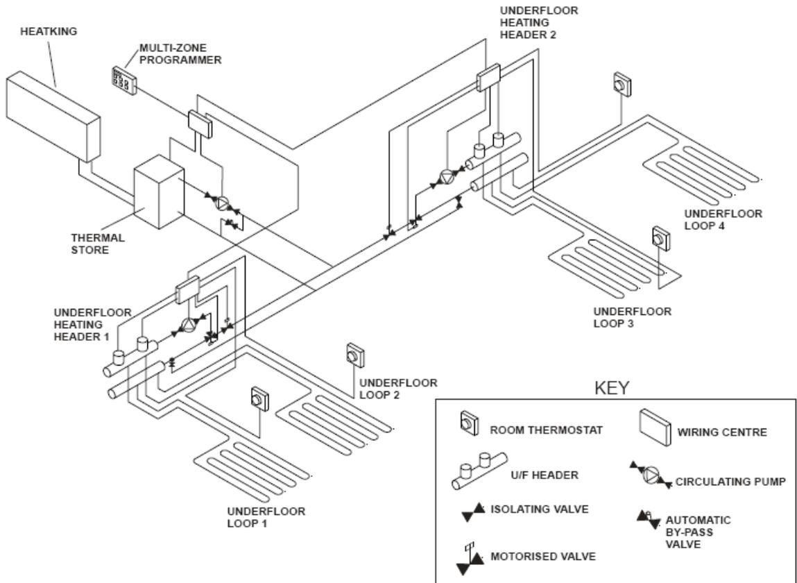
**Figure 74.** Underfloor Heating Diagram<sup>77</sup>
