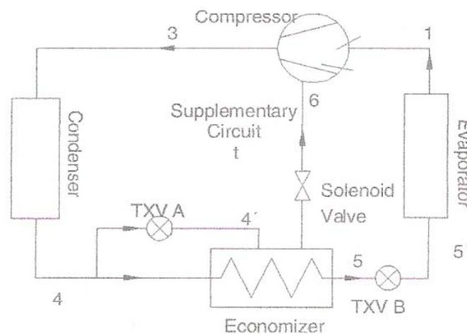
**Figure 8.** System Diagram- Principle of ASHP Improved Heat Pump Cycle <sup>21</sup>
