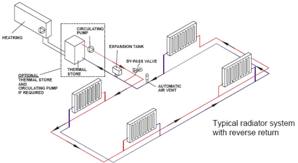
**Figure 73.** Radiator System Diagram<sup>76</sup>
