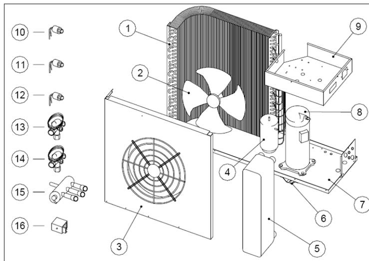
**Figure 22.** Exploded Diagram of Components <sup>70</sup>
