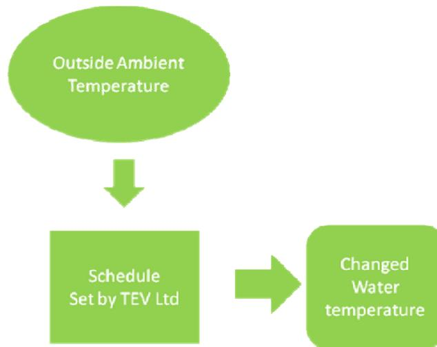
**Figure 34.** Compensation Flow Diagram
