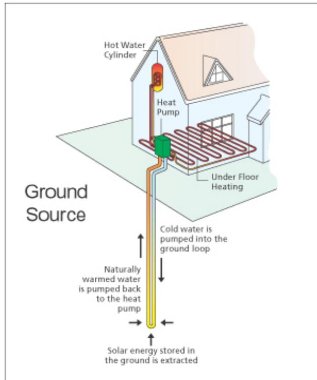
**Figure 1.** Ground Source Heat Pump Diagram <sup>4</sup>
