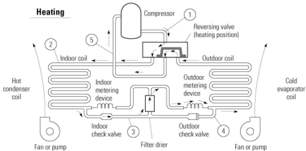
**Figure 5.** ASHP Component Diagram <sup>8</sup>
